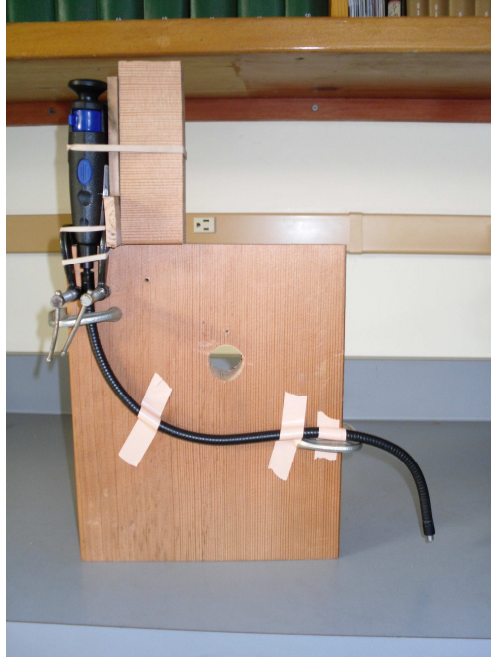
Figure 2. Borescope device and setup used for bench top laboratory investigation on detection accuracy for selected items. For digital images, the end of the fiber optic scope was adjusted to either 2 cm or 4 cm above the counter top. See the methods section for a complete list of materials included in the study for participant viewing.
