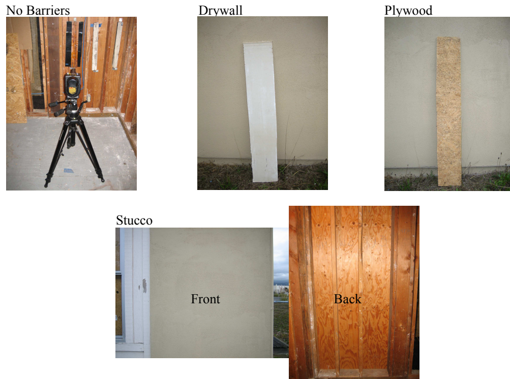
Figure 7. Wall coverings used to test the penetrating ability of X-ray and infrared to view damage and termites contained in field-collected boards. Test site, Villa Termiti Richmond, CA.
