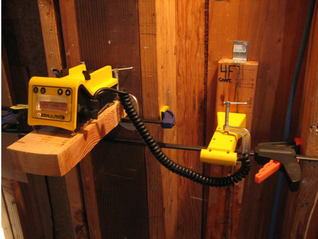
Figure 5. Test boards and portable microwave detection device used for field study. Test site, Villa Termiti Richmond, CA. The two yellow devices in the middle of the image are of a TERM_A_TRAC™ (Sidney, Australia). The left hand side device is the main operating component and the right side component is the sensor. Clamps were used to secure sensor to test boards.
