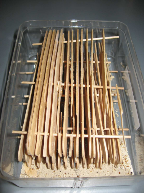
Figure. 2. Termite containment unit for collecting fecal pellets from Incisitermes minor (Hagen) workers.
